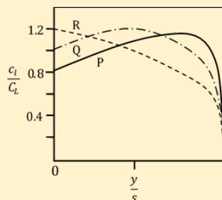
In the above figure,  $c_l$  refers to the section lift coefficient,  $C_L$  refers to the lift coefficient of the ring,  $y$  is the coordinate along the span and  $s$  is the span of the wing. A designer prefers to use a wing for which the stall begins at the root. Which of the wings will he choose?
